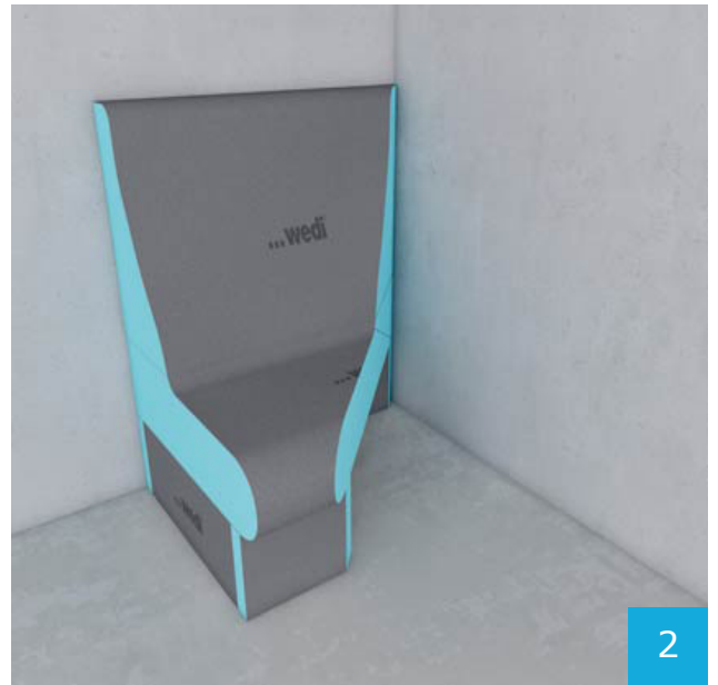
When using benches without corner elements, these should be mitred.
